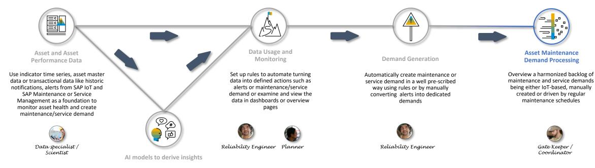
Leverage AI models like anomaly detection or Weibull algorithm to derive insights such as an anomaly score or probability of failure
